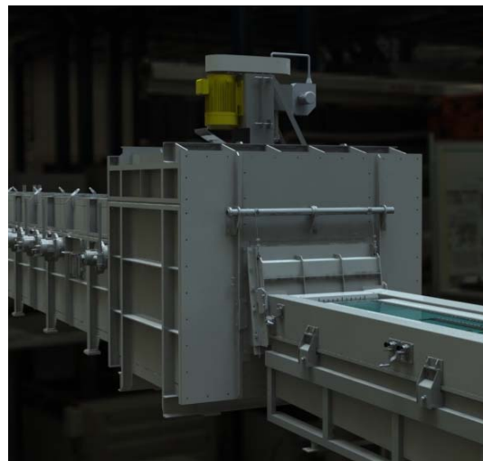
Recirculation fan drive (pat. pend.)
